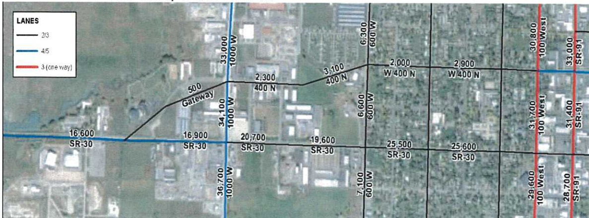
Figure 4: 2040 RTP Model without Western Arterial and with Jail Split and 400 North as 3-lane Collector to 100 West – Daily Traffic Volumes
